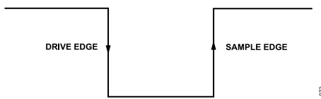
Figure 72. SPI Mode 3, SCLK Edges
